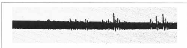
Figure 9b. Rib pattern: Ca = 35.3 ; V_m/V_t = 0.06 ; Re_m = 0.80 .
