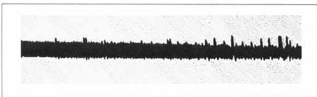
Figure 9c. Rib pattern: Ca = 9.6 ; V_m/V_t = 0.06 ; Re_m = 0.80 .
