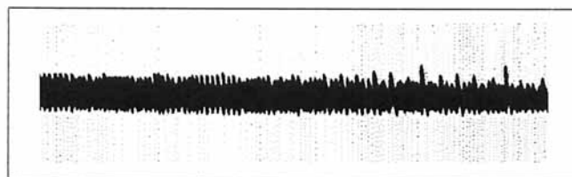
Figure 8b. Rib pattern: Ca = 8.5 ; V_m V_t = 0.03 ; Re_m = 0.38 .
